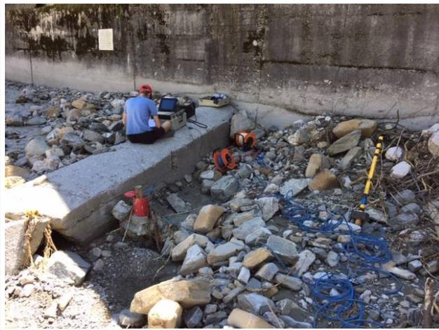
Profilo sismico down-hole2 (DH2) su sond. S2
