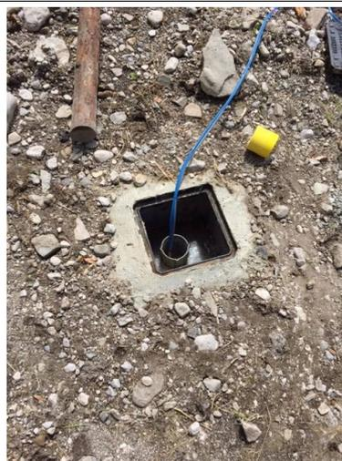
Profilo sismico down-hole2 (DH2) su sond. S1
